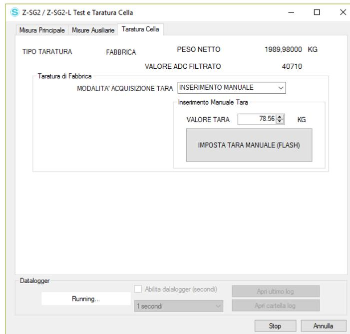
In Manual calibration mode, proceed as follows for calibration:
