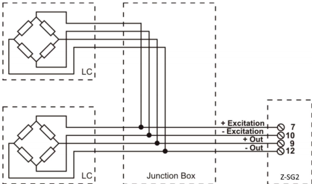
To connect 2 or more 6-wire cells in parallel with the SG-EQ4 junction box use the following diagram:
