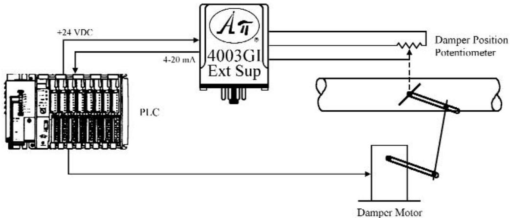
The external supply modification uses the +24 VDC power supplied by the PLC and regulates the 4-20 mA signal. The 2000 VRMS isolation protects against unexpected ground loops and electrical noise.
