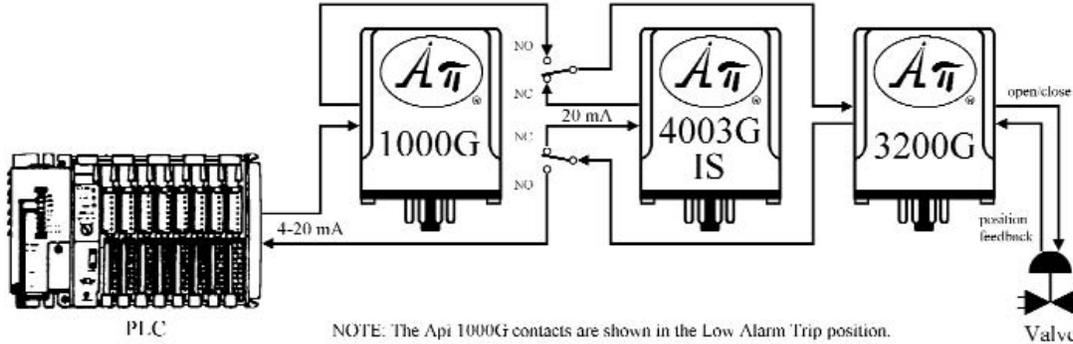
If the signal from the PLC drops below 4 mA, the **API 1000 G** will trip to a low alarm state, and select the 20 mA signal for the **API 3200 G**, thus commanding the valve to open fully. When the signal from the PLC is 4 mA or greater, the **API 1000 G** selects the PLC output signal for the **API 3200 G**, thus controlling valve position as normal.
