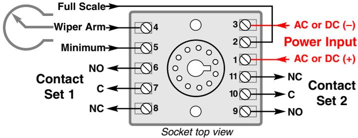
**Relay Output Terminals** – Terminals 6, 7, 8 and 9, 10, 11 provide the appropriate connections for the desired relay operations. (NO = Normally Open, NC = Normally Closed, C = Common). NOTE: Although the API 1800 G has a pair of relays, these relays will energize and de-energize in unison. The API 1820 G will accommodate independent relay operations.
