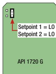
API 1720 G Internal Alarm Configuration Jumpers
