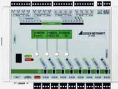
System to reduce power peaks, extendable in steps from 8 to 64 optimising channels.
