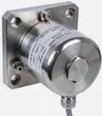
The KINAX N702-INOX HART is a very robust, absolute inclination transmitter. It is particularly suited for harsh environments due to its high mechanical strength and the hermetically sealed stainless steel housing.
