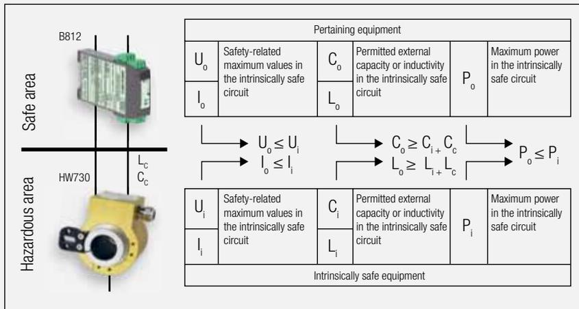
Test criteria of an intrinsically safe circuit using the examples of B812 and HW730
