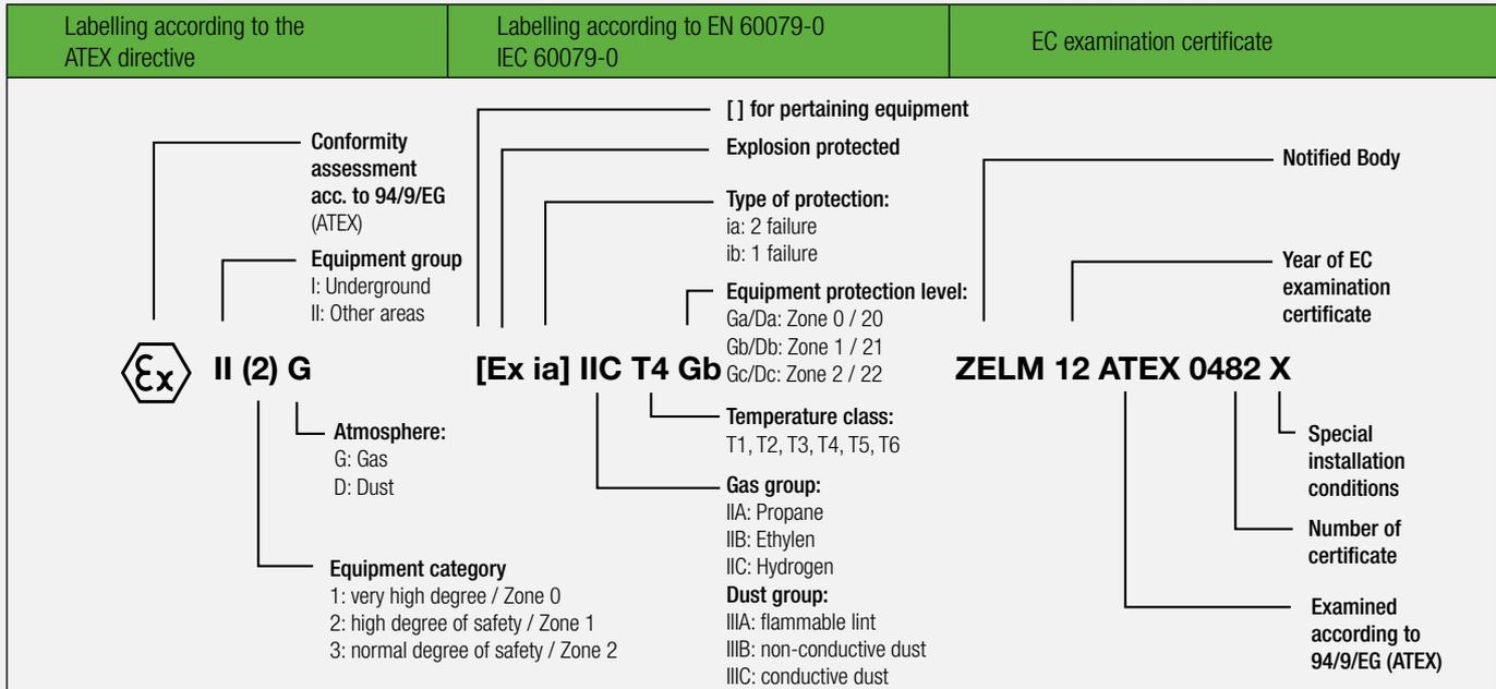
Labelling for electrical equipment according to IECEx
