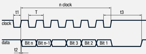
transmission of a complete data word requires n+1 rising edges (n = resolution in bits), e.g. 14 clock signals for a complete readout of a 13 bit encoder. After the last positive edge of the clock signal, the data line remains on low for t3 until the encoder is ready for a new data word. The clock line must stay just as long on high and can subsequently start a new read-out sequence of the encoder with a trailing edge.
