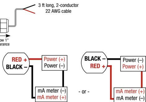
If the 4-20 mA analog output is not required, the transmitter will function as a low voltage powered temperature indicator when connected to any 8 to 32 VDC power supply. Connect the loop (+) supply to the RED lead and the loop (-) supply to the BLACK lead.
