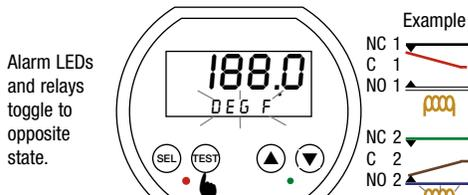
To exit the Alarm Test Mode, press and release the SEL button. The display briefly indicates - - - - and then returns to normal operation.
