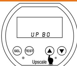
To change from upscale burnout to downscale burnout, press and release the ▼ button. The lower display will change to DN BO.
