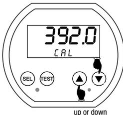
Use the ▲ and ▼ buttons to adjust the upper display segments to indicate the applied temperature value.
