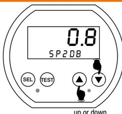
Press and release the SEL button to move on to the next parameter.
