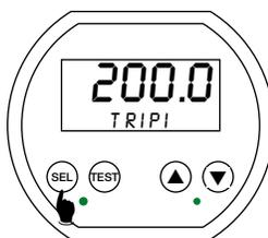
When the Trip Point 1 value is being displayed, press and release the SEL button. The Trip Point 2 value will be displayed with TRIP2 on the lower display.
