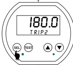
When the Trip Point 2 value is being displayed, press and release the SEL button. The RTD temperature will be displayed.
