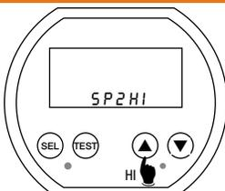
To configure Setpoint 2 as a Low Alarm, press and release the ▼ button. The lower section of the display will indicate SP2LO.
