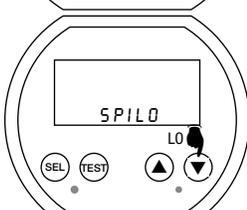
Press and release the SEL button to move on to the next parameter.
