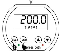
Release both buttons when the display indicates - - - -.
