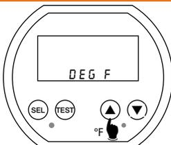
To change from degrees Fahrenheit to Celsius, press and release the ▼ button. The lower display will change to DEG C.
