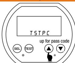
To disable Test and Set Point Adjust Mode pass code protection, press and release the ▼ button. The lower section of the display will indicate NOTPC.
