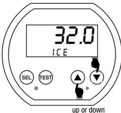
Use the ▲ and ▼ buttons to adjust the upper display segments to indicate 0.0°C or 32.0°F.
