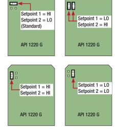
API 1220 G Internal Alarm Configuration Jumpers
