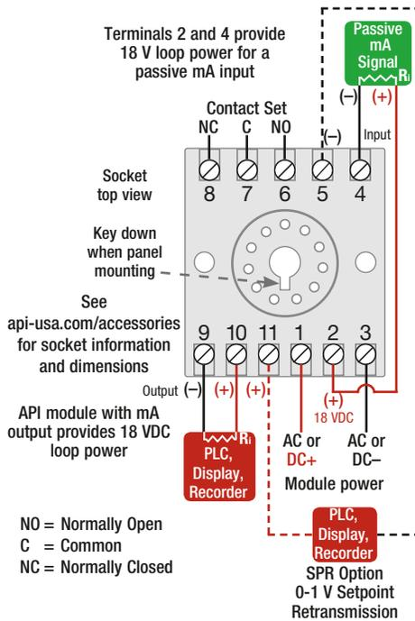
API 1040 G Using +18V Loop Power Supply
