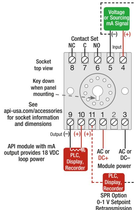
API 1040 G with Powered Current or Voltage Input
