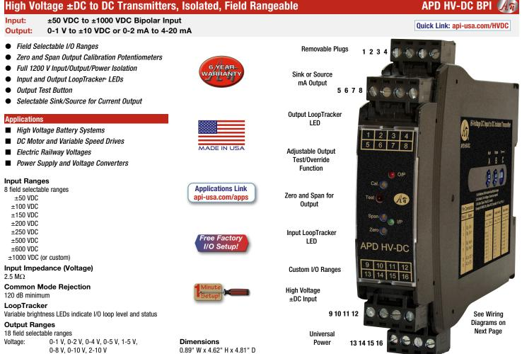
Bipolar voltage: ±5 V, ±10 V (recommended output) 0-2 mA, 0-4 mA, 0-8 mA, 0-10 mA, Current: 2-10 mA, 0-16 mA, 0-20 mA, 4-20 mA 20 V compliance, 1000  $\Omega$  at 20 mA
