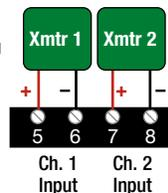
\* To avoid damage to the module, do not make any connections to unused terminals
