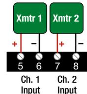
\* To avoid damage to the module, do not make any connections to unused terminals
