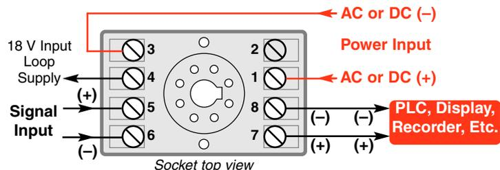
API 4050 G typical output wiring
