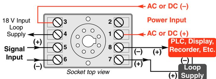
API 4050 G EXTSUP typical output wiring
