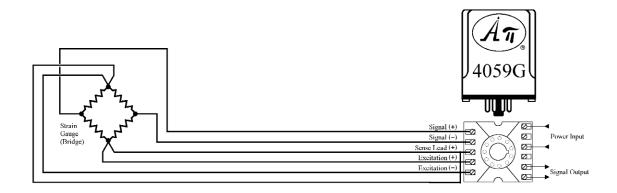
The API 4059 G Isolated Strain Gauge Signal Conditioner accepts a Sense Lead input. Internal circuitry in the module monitors the voltage drop in the bridge leads and automatically compensates the excitation voltage at the module so the actual excitation voltage at the bridge remains constant. Due to the design of the API 4059 G, it is only necessary to connect one of the sense leads for the feature to be effective.
