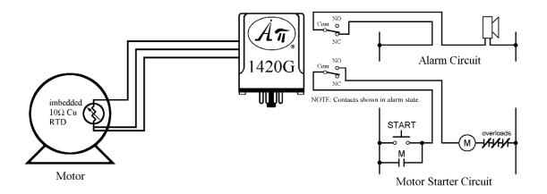
Setpoint 1 is adjusted to the rated temperature, and Setpoint 2 is adjusted to the rated temperature plus 10 degrees. The standard heavy-duty relay contacts are rated 7A @ 240 VAC and can directly control most devices.
