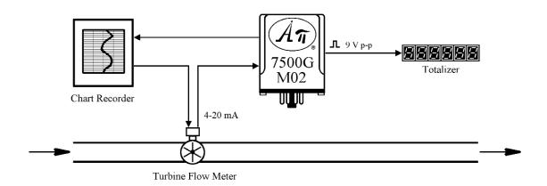
The API 7500 G M02 provides the 9 V p-p square wave required by the totalizer system.
