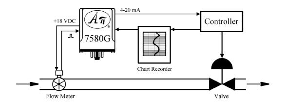
The **API 7580 G** features 30 selectable input ranges from 0-100 Hz to 0-30 KHz, and 16 selectable output ranges. In addition, the optical isolation protects against unwanted ground loops and electrical noise.
