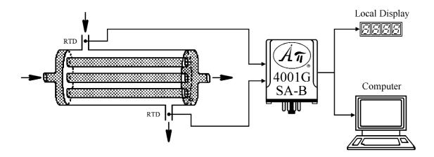
The API 4001 G SA-B will directly measure the temperature differential and provide an output to drive the local display and the process control computer.
