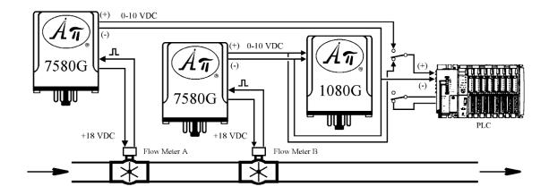
The second set of relay contacts of the **API 1080** G provides a PLC binary input with a closure to indicate which flow meter is selected.
