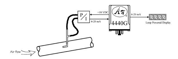
Since Flow = Velocity x Area, the cross sectional area of the pipe will determine the range of the scaling on the loop powered display. This allows the velocity value to be displayed as a flow rate. The optical isolation of the module protects against unwanted ground loops and electrical noise.
