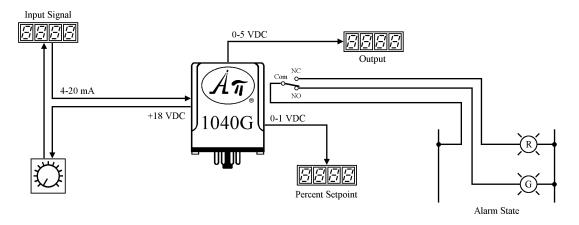
The Api 1040G SPR option provides a 0-1 VDC transmitted signal indicating the location of the setpoint in percent of span.
